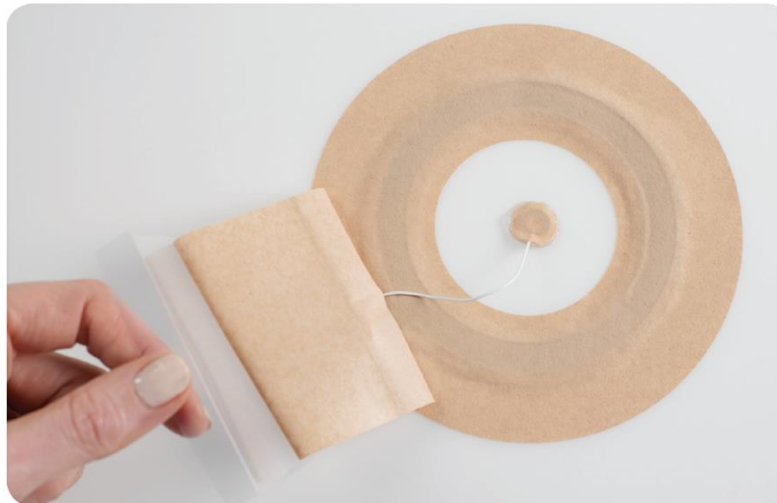
Figure 5: A photo of an electroceutical, wound therapy bandage. A flap is pulled back to reveal the central cathode on the wound viewing window which is connected in series to the outer anode [31]
