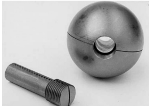
Figure 1.4: Non-fissile instrumented melt wire pebble for measuring temperatures in the AVR [60].
