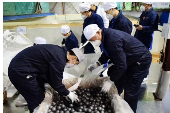
(b) Pebble fuel under inspection
