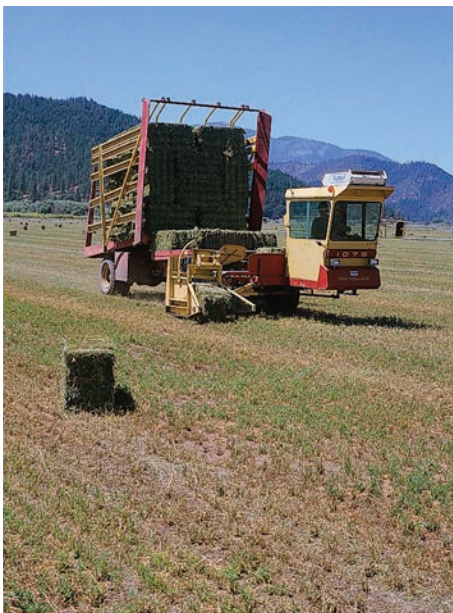
Small bales averaging about 125 pounds are collected in a bale wagon in Scott Valley (Siskiyou County).
