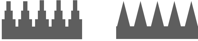
Figure 4.38: A cartoon drawing of the cross section of the metamaterial. Left: the cross section of the metamaterial from the step dicing. Right: the cross section of the pyramid-shaped metamaterial.
