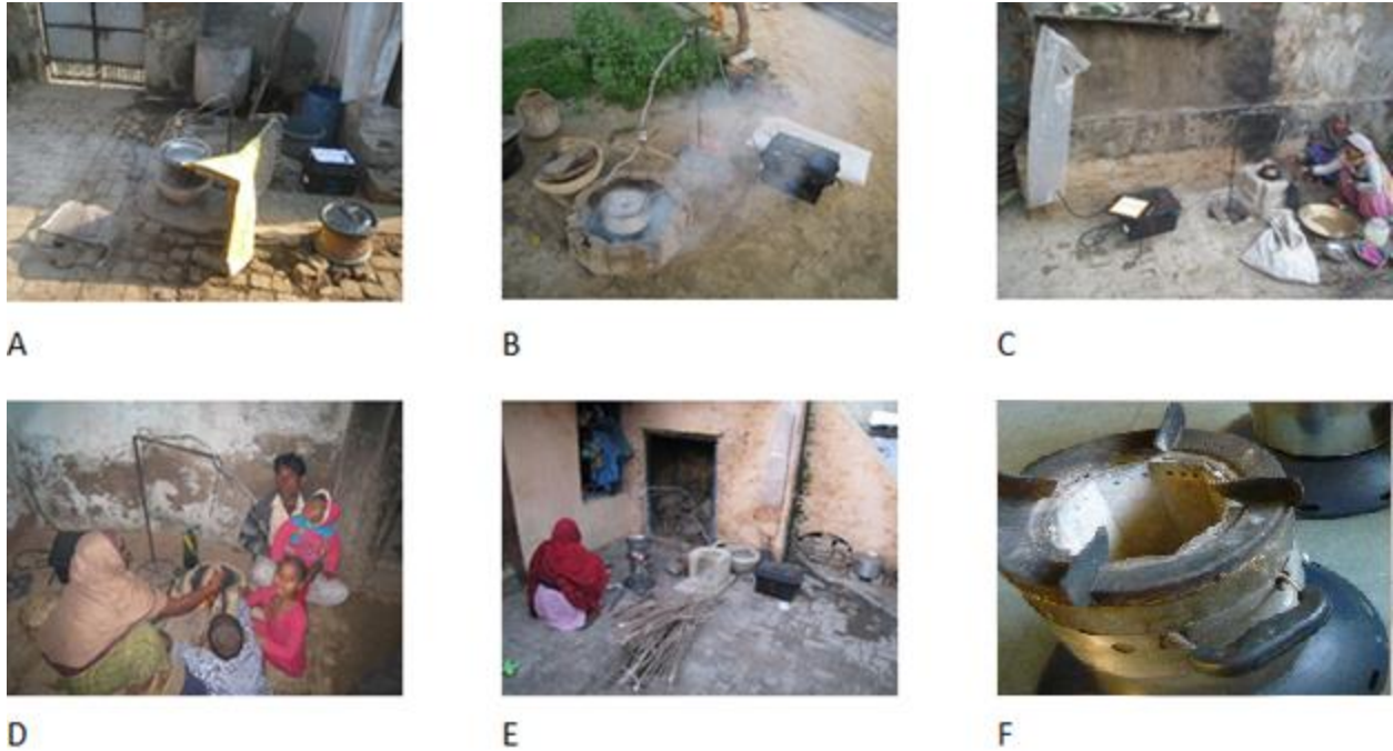
Figure 1.1: Pictures of all stoves tested. The Haro, a portable Angithi, filled with smoldering dung during emissions sampling (A), a fixed Angithi utilizing smoldering dung to cook animal feed (B), a fixed Chula and sampling equipment pictured before emissions began (C), a fixed Chula loaded with brushwood pictured during indoor cooking of bread (D), a Philips stove loaded with brushwood during outdoor cooking (E), and a close-up of a used Philips stove (F).
