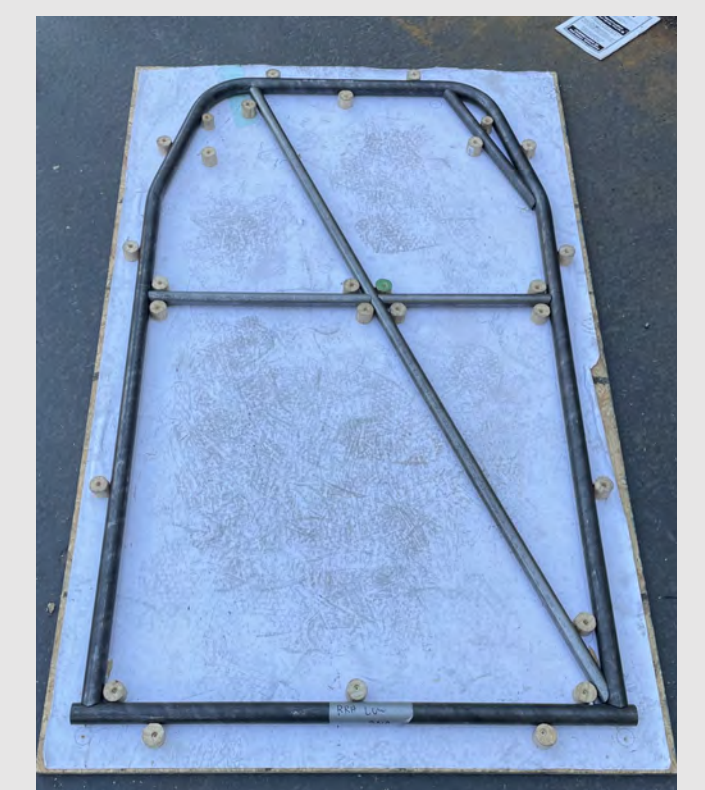
Figure 7: Manufactured Rear Roll Hoop In 2D Jig
