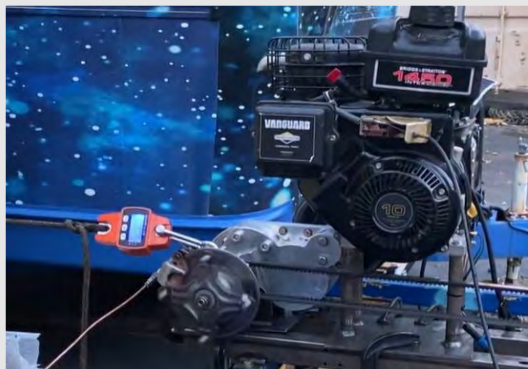
Figure 1: Dynamic Torque Testing Done with Vanguard Engine
