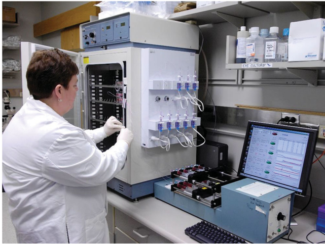
FIGURE 6. Perfusion system in the Fautsch Laboratory at Mayo Clinic (Rochester, MN). Shown is a humidified, 37°C, 5% CO 2 incubator with PE60 tubing connecting the flow chambers to the syringe pump (blue box) and to a pressure transducer (on the right outside the chamber). It is notable that a tray/pan of water with antibacterial such as Lysol placed in the bottom of each incubator and changed regularly is essential to maintain 100% humidity and to avoid evaporation errors. The monitor indicates pressure transducer readings.
