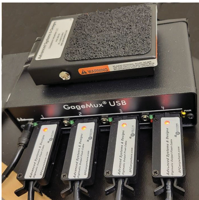
FIGURE 10. GageMux USB with foot pedal to initiate readings and four USB connections to read the four balances. Data are inserted into an Excel file on a connected laptop.
