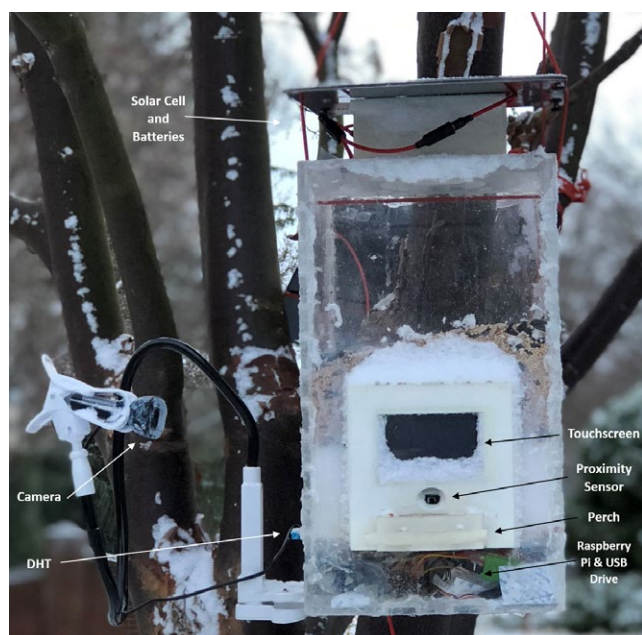
FIGURE 1 The PASSER smart feeder with key components labeled
