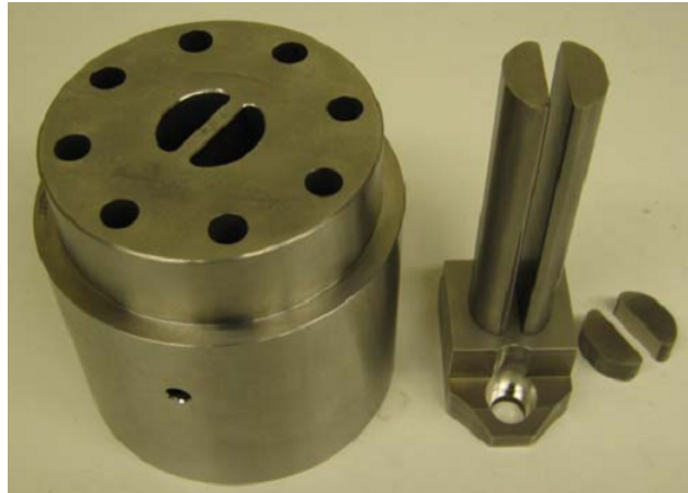
Figure A.2: Form left to right: container, ram-stems and dummy-blocks.
