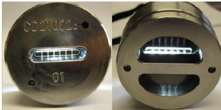
Figure A.1: Extrusion die.
