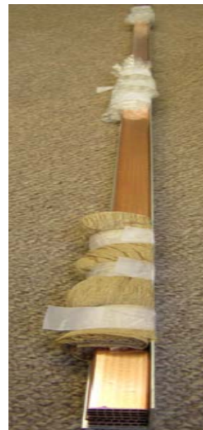
Figure A.11: Tubes packed with aluminum angle supports for shipment.
