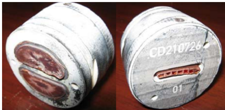
Figure A.12: Residual copper in the container and die.
