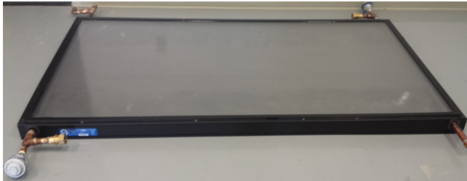
Figure 2.15: The copper minichannel absorber placed inside a commercial metal frame (1021.1 mm by 1935.5 mm) made for conventional solar flat-plate collectors.
