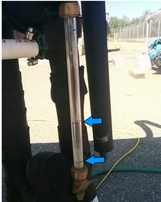
Figure 5.8: Tracking the steam generation rate by marking the sight glass with the start and end fill lines, and timing the steam generation as the water level at the end line drops to the start line.
