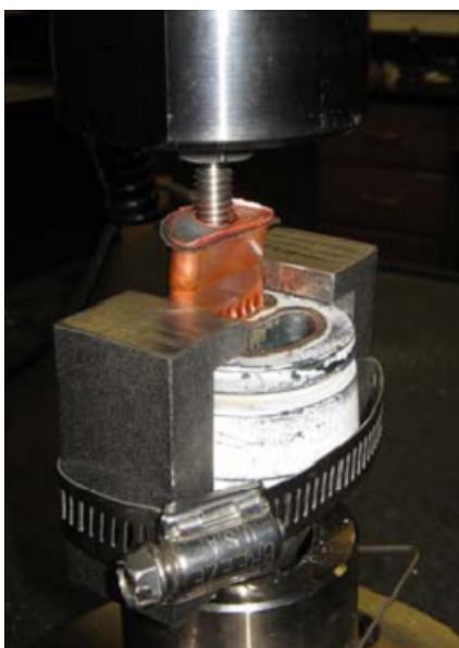
Figure A.13: The Instron® machine removing the residual copper from the container.
