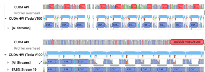
Figure 5. Timeline of CG (top) and CGAsync (bottom) on rank 2. Each ran ten iterations. The blue csr... bars are csrMV (i.e., SpMV ) kernels in cuSPARSE, and the red c... bars are cudaMemcpyAsync() copying data from device to host.
