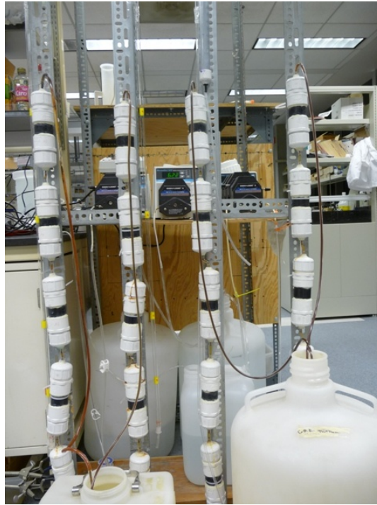
Figure 4.1 Picture of the column setup used for the determination of the effect of carbonate on the hydraulic properties of the ZVI bed.
