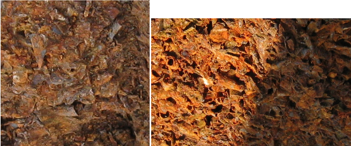
Figure 3.18 Close views of ZVI taken out of the reactor when it was dismantled showing the heavy deposits of iron corrosion products and quasi total loss of porosity.
