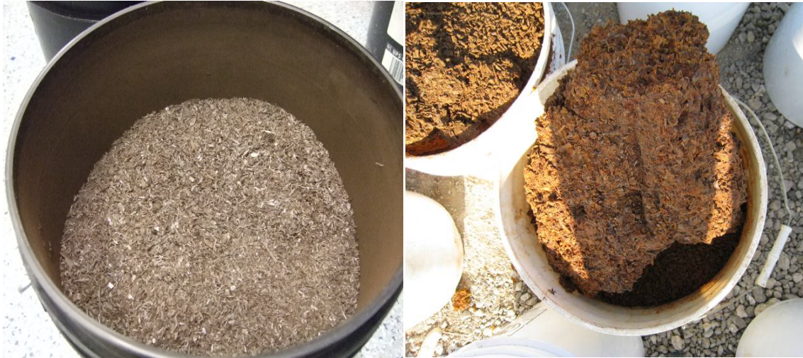
Figure 3.17 Pictures of fresh ZVI (left) and large blocks of ZVI (right) taken out of the reactor when it was dismantled showing the solid structure of the ZVI bed.
