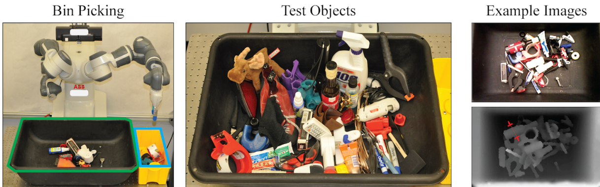
Figure 5.3: Experimental setup for benchmarking bin picking policies. (Left) For each experiment, a subset of N validation objects are randomly dropped into a bin (green rim, center), at which point the YuMi iteratively plans grasps from point clouds and attempts to lift and transport the objects to a packing box (blue rim, right side). (Middle) A set of 50 test objects with various shapes, sizes, and material properties. A subset of 25 are rigid and opaque, and 25 others have transparency (e.g. goggles), moving parts (e.g. can opener), or deformable material (e.g. cloth). (Right) Example color and depth images from the physical setup with example grasp planned with the Dex-Net 2.1 \epsilon = 0.9 policy.
