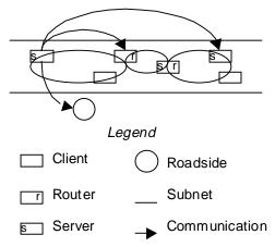
Access to IP addresses outside the AHS (and in general to Internet protocols) could also be provided, through the road-side. This allows vehicle occupants to read/write e-mail, browse the net, etc. Of course such activities must be assigned a limited amount of bandwidth to make sure they don't interfere with AHS operations.
