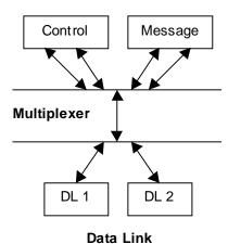
The control component of the network layer contains a subnet manager to handle subnet operation and a routing manager to allow messages to be sent through different subnets. The control component of the transport layer contains a QOS manager to ensure that a user-specified QOS is provided when transmitting data.
