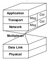
The (de)multiplexing layer is needed to direct messages coming from a data link layer component to the message or control part of the network layer and viceversa.
