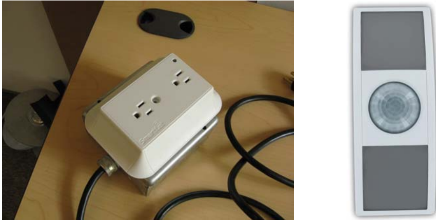
Figure 3: Controlled Receptacle (mounted on receptacle with extension cord) and Occupancy Sensor (Technology Package 1)
