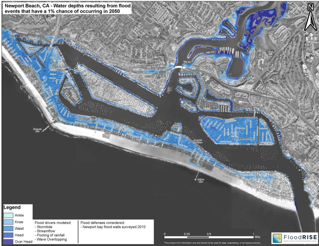
Map C. FloodRISE 1% AEP depth in 2050 - This map predicts what the flood depths from 1% AEP flood events in 2050 will look like. To model the 1% AEP of sea level for this scenario, sea level rise predictions from the National Research Council for the southern California coast were aggregated with an analysis of sea level variance based on 91 years of stormtide measurements recorded at NOAA's Los Angeles tide gauge (ID: 9410660).
