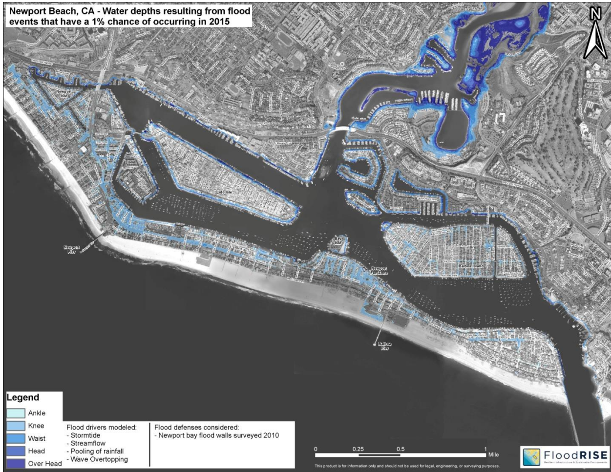
Map B. FloodRISE 1% AEP depth in 2015 - This map shows the water depths resulting from flood events that have a 1% chance of occurring in 2015. The flood drivers considered during hydrodynamic analysis are stormtides, wave overtopping along the Balboa Peninsula, runoff and pooling from rainfall, and streamflow into the Newport Bay from the San Diego Creek, Bonita Canyon and the Delhi channels (not shown in map). The flood heights are related to body height as shown in the legend.
