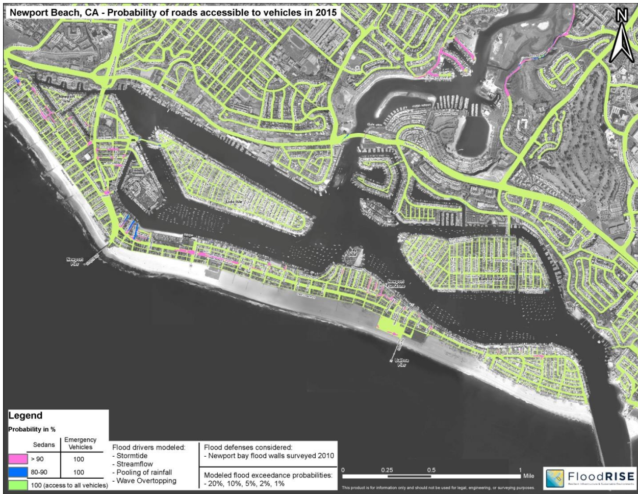
Map F. FloodRISE roads accessible to vehicles in 2015 - This map shows the probability of streets being accessible to sedans and emergency vehicles under current climatic conditions (2015). The flood depth threshold adopted to discern road accessibility to sedans is 18 inches (1.5 ft), while for emergency vehicles a depth of 30 inches (2.5 ft) was used. While some road segments have a low probability of becoming inaccessible to sedans, all roads remain accessible to emergency vehicles since current flood conditions in the Newport Bay are not capable of generating flooding along streets over 2.5 ft in depth.
