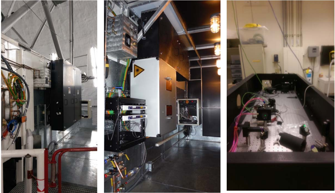
Figure 6: Left: The old dye laser amplifier table enclosure (the large rectangular unit in black). Middle: The new TOPTICA/MPBC laser (the white unit in the middle) and new laser table (black unit above the laser). The fiber splice boxes can be seen on the mid-left. The design of the laser head and new laser table allows the addition of two more lasers to support future AO upgrades. Right: The new laser table with fore-optics relaying the laser beam to the CLS.
