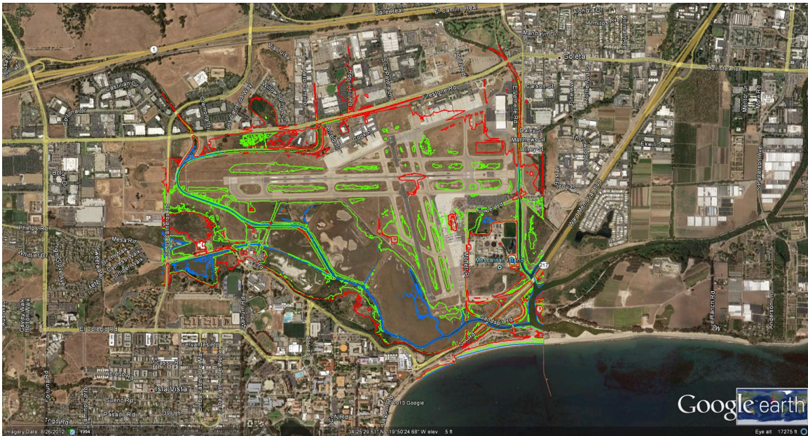
Figure 2.14 Projected future coastal flood inundation map for the Santa Barbara Airport using NOAA’s 2010 LiDAR data and Google Earth. Blue lines show the present mean high water level at 4.4 feet (1.35 meters). Green lines show extent of 100-year flood (3-ft flood) on top of 2 feet of sea-level rise (NRC’s most recent high sea-level rise projection relative to sea level of the year 2000) at high water, for a total elevation of 9.4 feet for the year 2050. Red lines show extent of 100-year flood (3-ft flood) on top of 5.5 feet of sea-level rise at high water for a total elevation of 12.9 feet for the year 2100.
