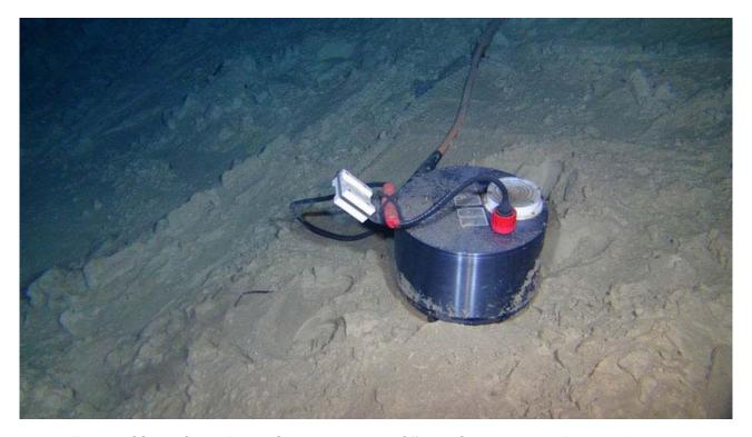
Figure 1. CSnet's Ocean Bottom Seismometer at the Offshore Communications Backbone's Node 4
