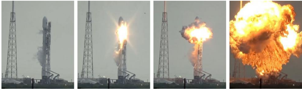
Figure 1-5 COPV failure caused the loss of payload, vehicle and damage to the launch facility during SpaceX Sep 1 2016 pre-launch (Image: US Launch Report).
