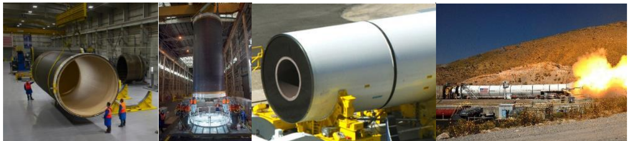
Figure 1-6 (L) Empty composite segment case (Image: Airforce-technology.com), (ML) prepare for hydro-pressurize test (Image: Spaceflight Insider) (MR) Segment after solid fuel casting (Image: nasaspaceflight.com), (R) Static fire test (Image: Northrop Grumman Newsroom).
