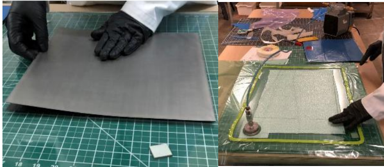
Figure 4-3 The Ti plies have slight curvature and does not adhere to composite plies well and a debulking step (apply vacuum pressure) is added
