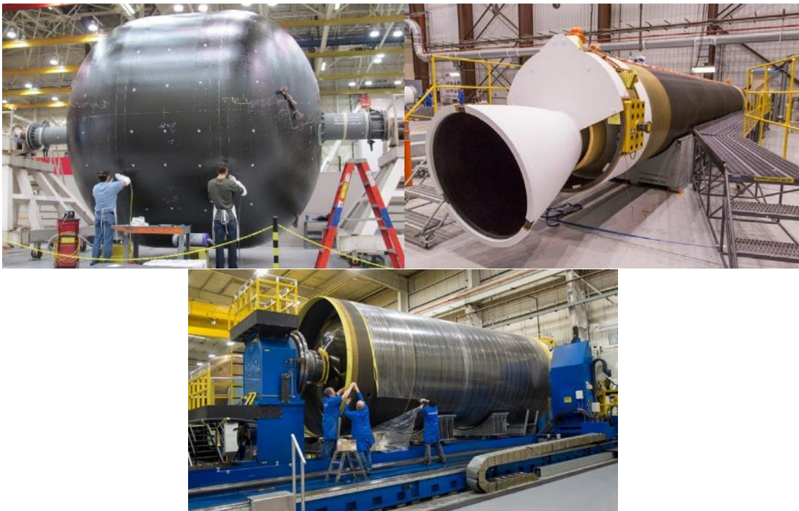
Figure 1-4 (L) Composite overwrap pressure vessel (Image: structures.aero). (R) Graphite epoxy motor (Image: spaceflight101), (B) Filament wound composite pressure vessel (Image: AIAA.org)
