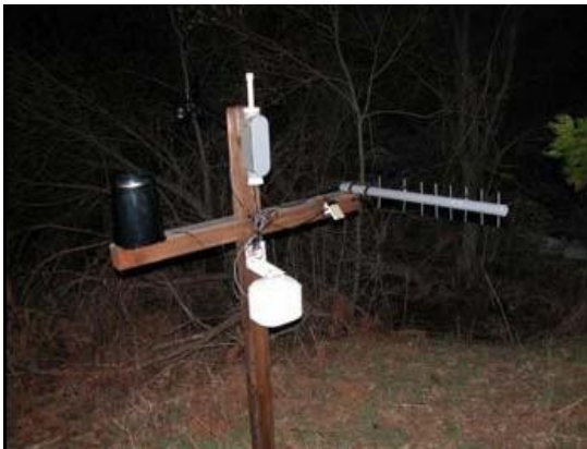
Figure 2.1: CMS micro-climate station
