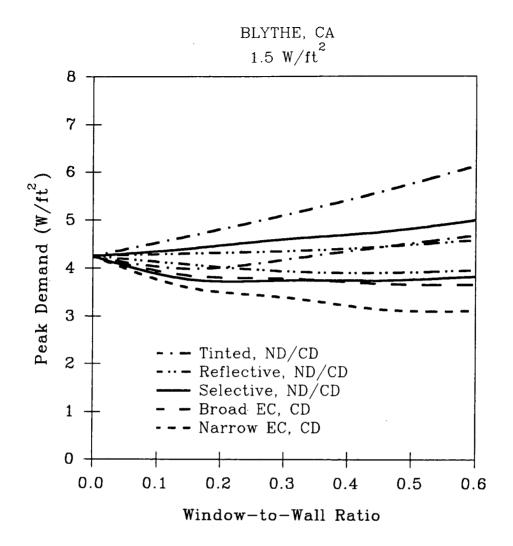
Figure 7. Total Perimeter Zone Peak Electricity Demand for the Five Window Prototypes
