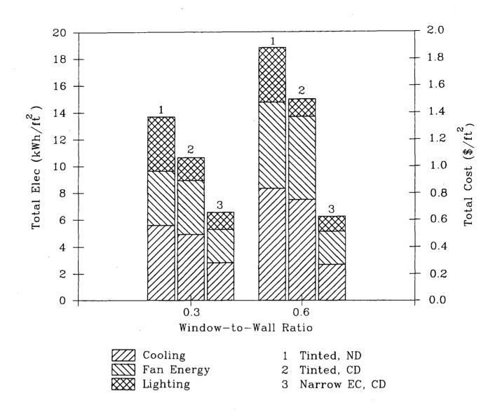
Figure 9. Annual Electricity Consumption and Cost by Load Component for Selected Window Prototypes in the West Perimeter Zone
