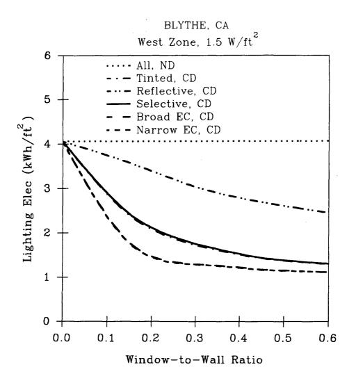
Figure 3. Annual Lighting Electricity Consumption for the Five Window Prototypes in the West Perimeter Zone
