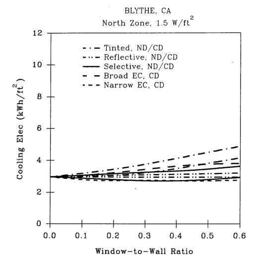
Figure 5. Annual Cooling Electricity Consumption for the Five Window Prototypes in the North Perimeter Zone
