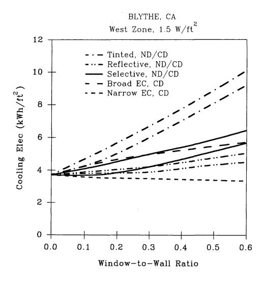
Figure 4. Annual Cooling Electricity Consumption for the Five Window Prototypes in the West Perimeter Zone
