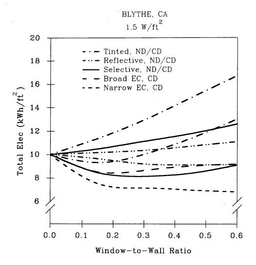
Figure 6. Total Perimeter Zone Annual Electricity Consumption for the Five Window Prototypes
