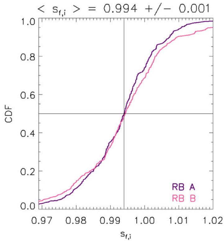
**Figure 4:** Cumulative distribution function (CDF) for the appropriate value of the shorting factor  $s_{f,i}$  for Van Allen Probes A (RB A, in purple) and Van Allen Probes B (RB B, in pink). The median value for  $s_{f,i}$  is 0.994, and the standard error of the mean is of 0.001.
