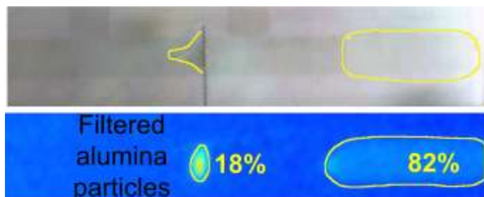
Figure 4.10: (A) Visible light image capture of droplet after filtration of alumina particles. (B) Cerenkov image, showing purified product droplet (right) and alumina-containing droplet (left).
