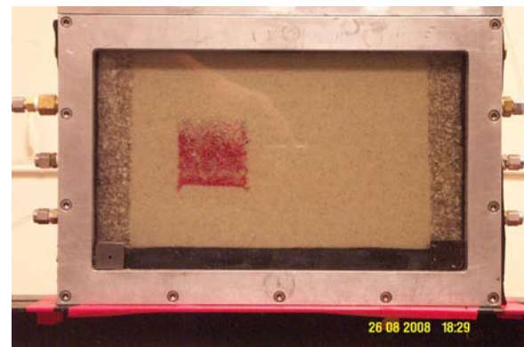
Figure 1. Two-dimensional flow cell used in the experiments. The total length of tank is approximately 30 cm and the DNAPL source zone (red) is 5x5 cm.
