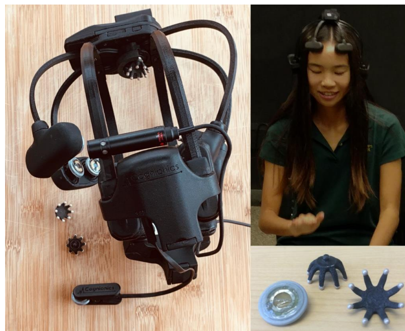
Figure 2. Left: Cognionics headset used for the present study (viewed from the left); right top: a research assistant tests the headset and drum machine; right bottom: tined and smooth electrodes for placement in hair and on the skin, respectively.
