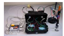
System w/circuit boards designed to make mini-sensors compatible with commercial data logger
