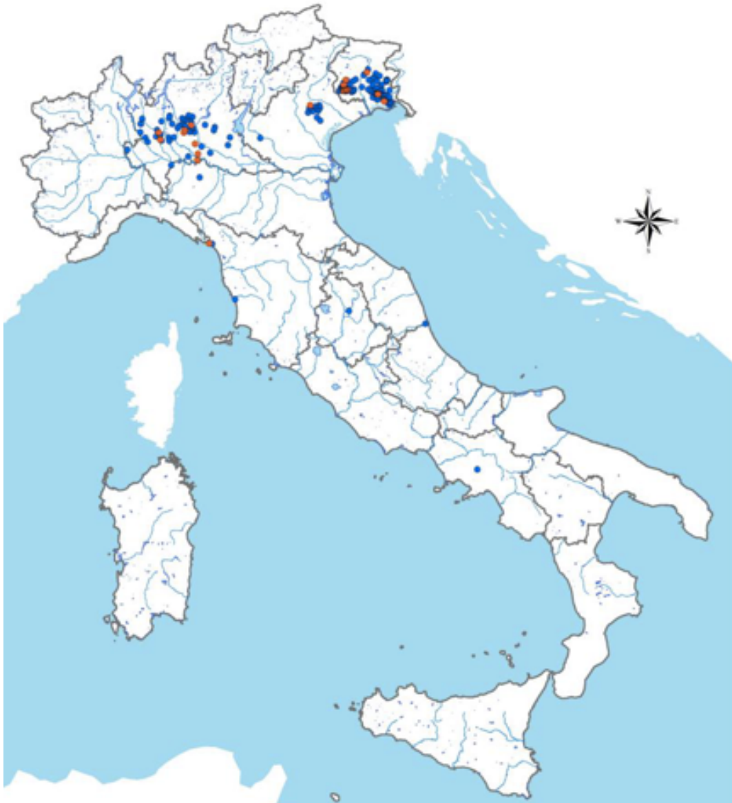
Figure 8. Groundwater contamination with atrazine and atrazine metabolites in 2012. Red dots represent where atrazine was found above 0.1 µg/L and blue dots represent atrazine concentrations below 0.1 µg/L. Source: ISPRA, 2014.
