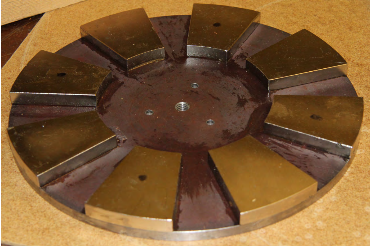
Figure 4.1: One disc of the magnet rotor. The full rotor is assembled with two facing discs.
