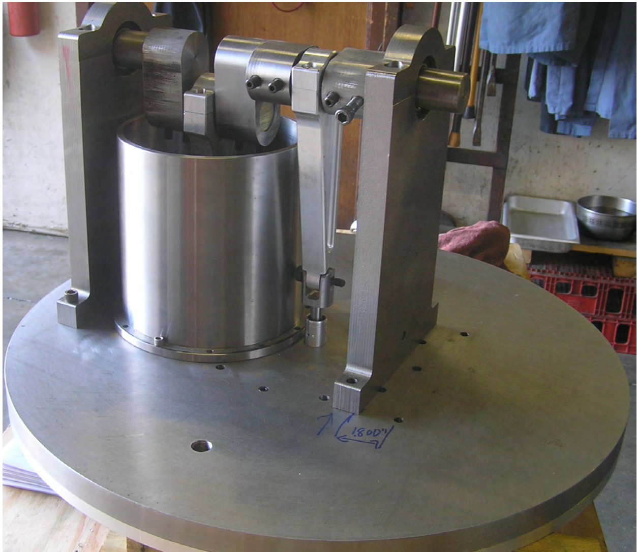
Figure 3.14: Crankshaft assembled with connecting rods to pistons.
