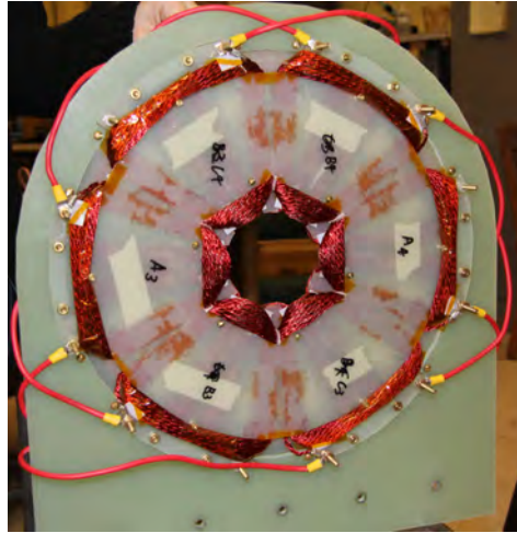
Figure 4.2: The assembled winding structure. The two winding halves were assembled facing each other on the support structure.
