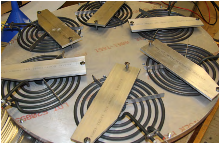
Figure 5.2: The electric heater assembly is shown here, bolted against the external side of the hot-side heat exchanger.
