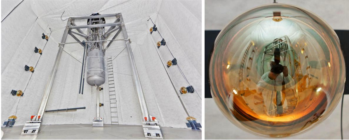
Figure 4.2: At left: wide-angle view of the LUX water tank interior. Three of the veto system vertical PMT strings are visible. Note also the gray, horizontal acrylic tube, which was raised during DD calibrations to allow neutrons to reach the TPC (see Sec. 3.4.3). At right: close-up of a Hamamatsu R7081 10" PMT, mounted at the lowest level of one of the four vertical strings.
