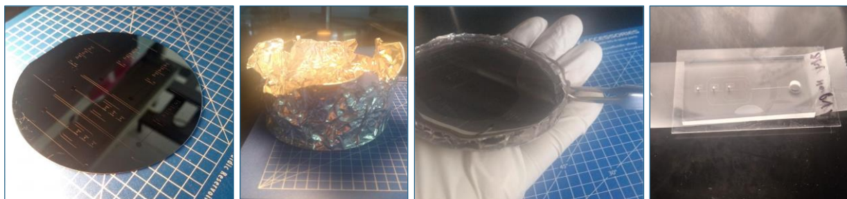
Figure 11. Images of PDMS microfluidic chip making process. Shows the silicon wafer, tinfoil wrap, removal of PDMS from wafer, and the finished PDMS chip on bonded to a slide.
