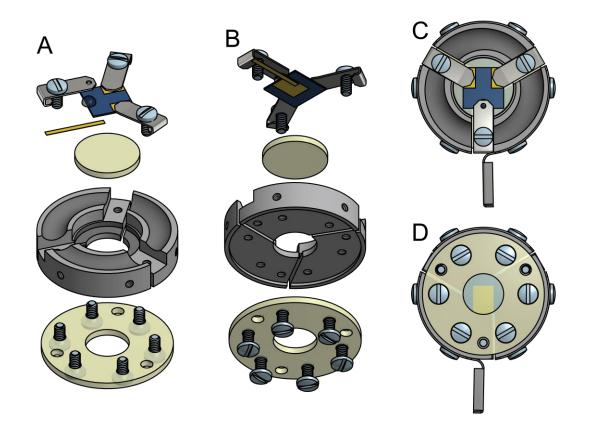
Figure B.3. Sample holder photos. (A) and (B) are the isometric views of a split sample holder from bottom right and top right respectively. This sample holder is not grooved and can be used for large 2D sample. (C) Top view of a sample holder with grooved ramps. (D) Normal sample holder with planar ramps.
