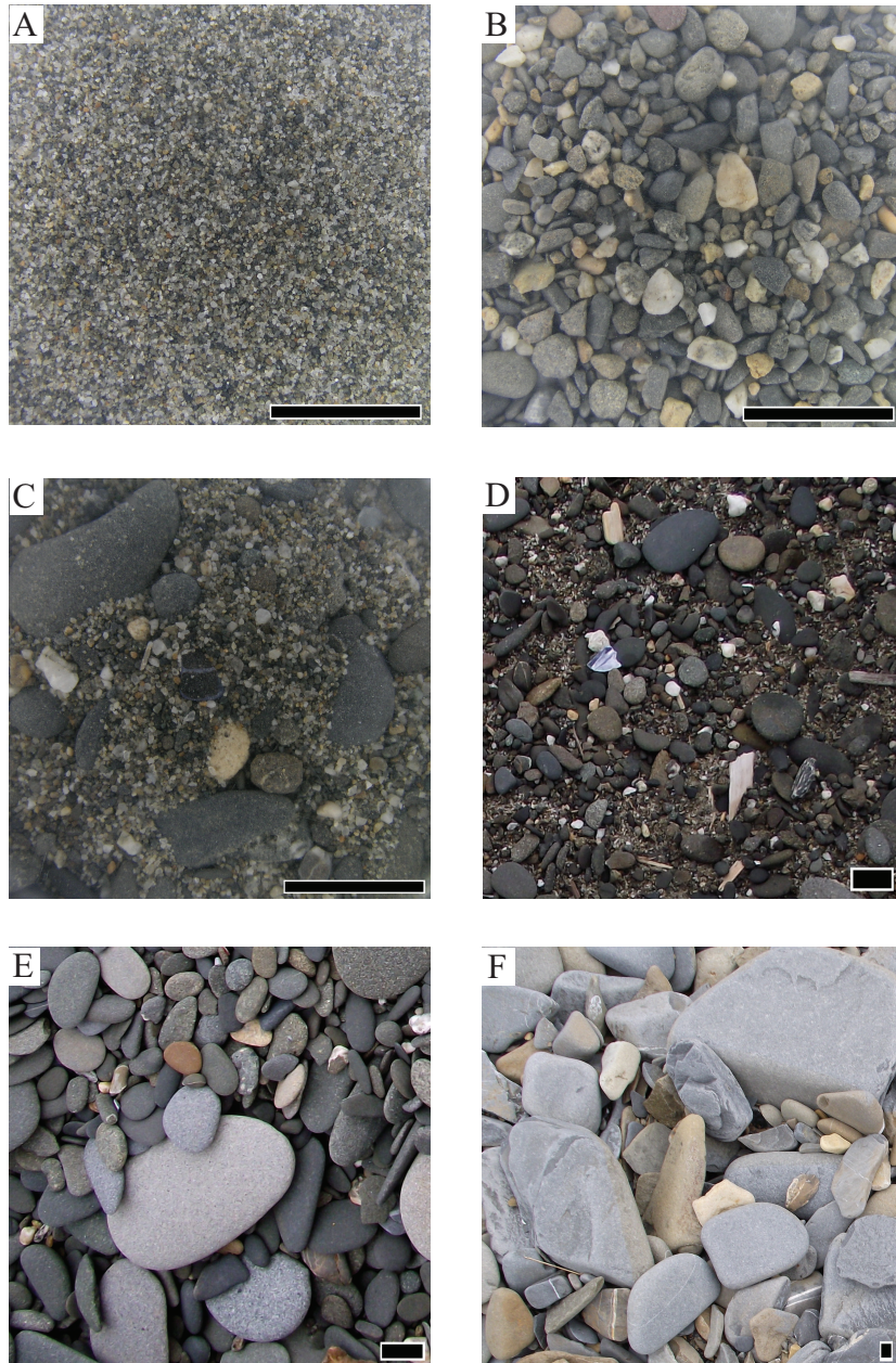
Figure 2.9. Sediment samples from Shaktolik's beaches. The black bar represents 1 cm. These images display the wide variations in grain size and sorting along the beaches. Mean grain sizes calculated: (a) 0.61 mm, (b) 2.48 mm, (c) 2.25 mm, (d) 4.02 mm, (e) 15.92 mm, and (f) 64.64 mm.
