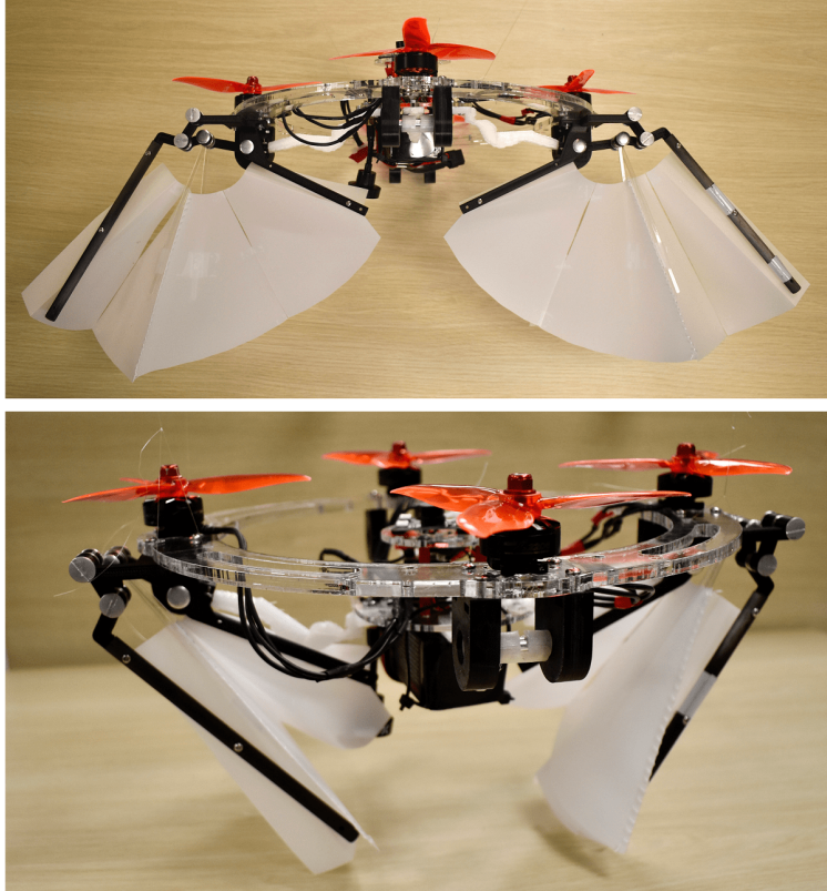
Figure 7.20: The fabricated HAV prototype with fixed wing (top) and quadrotor (bottom) modes.
