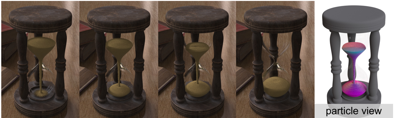
Figure 5.33: Hourglass. Sand in hourglass accumulates at the bottom. The material is modeled with Drucker-Prager plasticity (Klár et al., 2016).
