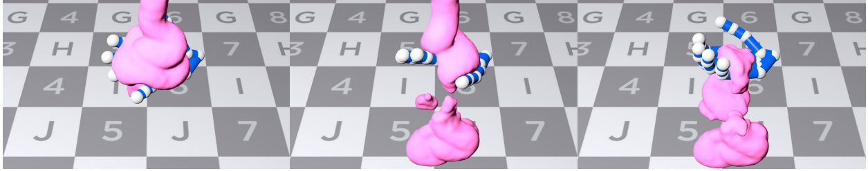
Figure 5.35: Real-time Vision Pro™ Interaction. Interactive manipulation of a viscoelastic fluid, consisting of up to 20K particles, is simulated at 30fps.
