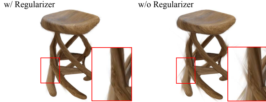
Figure 6.19: Anisotropy Regularizer. We introduce an anisotropy constraint for Gaussian kernels, effectively enhancing the fidelity of the Gaussian-based representation under dynamic conditions.
