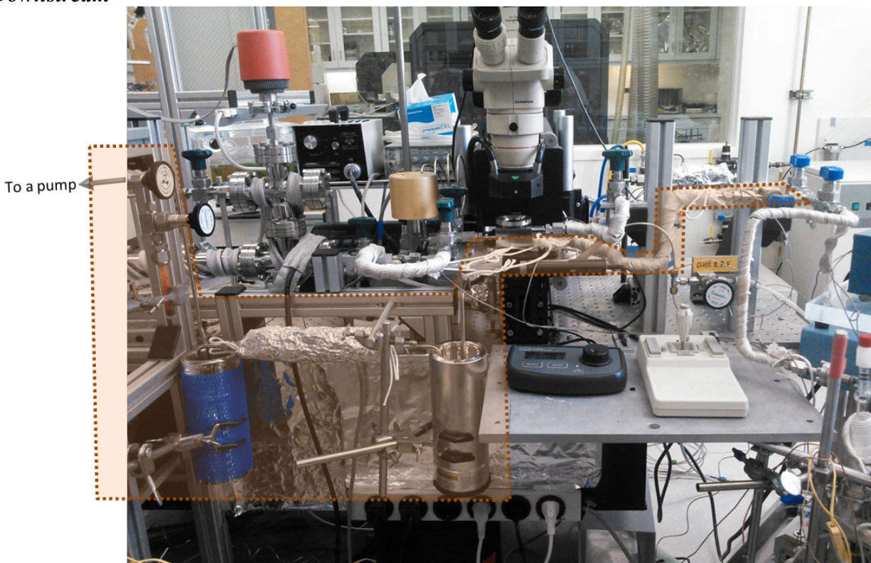
Figure 2-9. A picture of the vacuum extraction line of the Young laboratory laser fluoridation. The area indicated in brown is downstream section.
