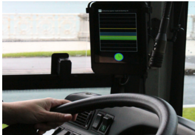
Figure 6.4: Installation of the on-board control equipment in Dbus, San Sebastián.
