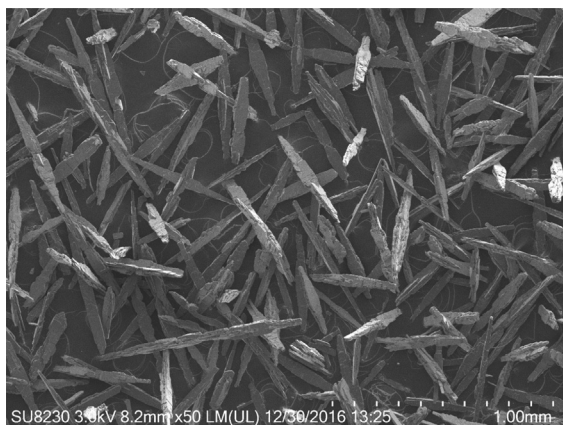
Fig. 5. SEM image showing representative anhydrite crystals from isotope exchange experiment A. The product anhydrite from both phase separation (not shown) and isotope exchange experiments are similar in size and morphology and therefore surface area is not explicitly accounted for in the rate law. The crystals show signs of dissolution and post experiment fracturing and therefore the original surface area is estimated as a right rectangular prism. See section 3.2 for details.
