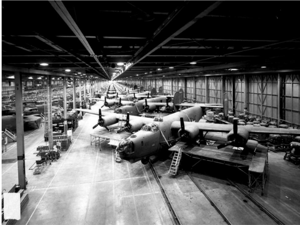
**Figure 4.3: General Motor’s Willow Run plant, named for the nearby creek, produced one B-24 bomber every hour during WWII. Architect Albert Kahn called this “the largest room in the history of man” (Corps 1940)**
