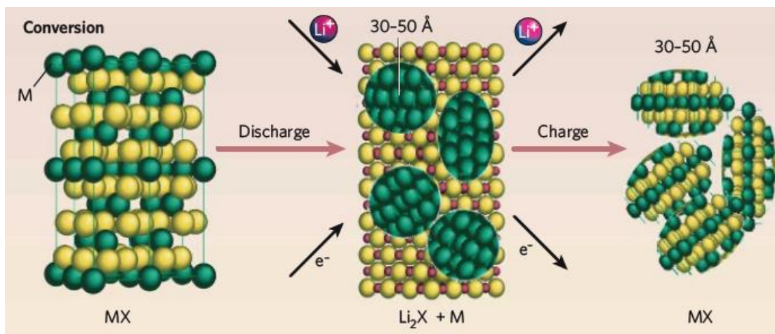
Figure 2.1 Schematics illustrating conversion mechanisms. The conversion reaction can transfer 2 to 6 electrons [14]
