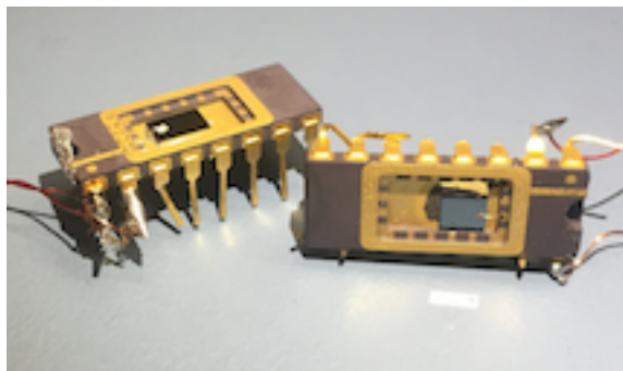
Figure 4.6: 16-pin dual in-line package chip carrier for QD samples.
