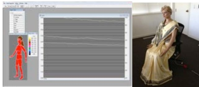
Figure 7. The manikin control screen (left), climate chamber and thermal manikin ‘Monica,’ in a sari
