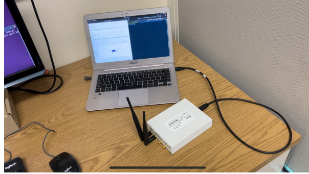
(b) The B210 plugged into the laptop via USB
