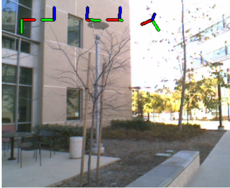
Figure 1.5: Relationship between 3D coordinate frames. Rendered along the top of the image are the coordinate frames relative to the image plane. From left to right are the camera coordinate frame, the pitch-roll-yaw rotated local Cartesian coordinate frame, pitch-roll-yaw unrotated local Cartesian coordinate frame, WGS84 local Cartesian coordinate frame, and WGS84 geocentric coordinate frame. For each coordinate frame, the X -axis is in red, Y -axis in green, and Z -axis in blue.
