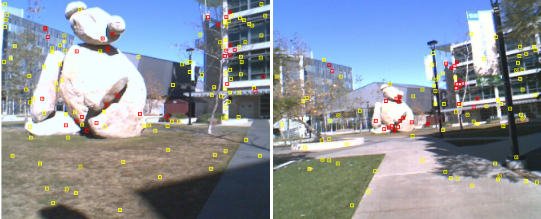
Figure 1.7: Features for matching. SIFT features (in yellow and red) detected in images acquired by two different cameras. 127 and 101 features were detected in the left and right images, respectively. A combination of guided matching, SIFT descriptor comparison, and robust modeling fitting is used to determine the set of feature correspondences between the two images—29 of these feature points are inliers (in red) and the remaining detected points are outliers (in yellow).
