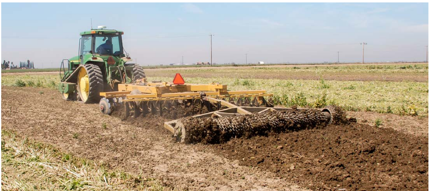
A disk plow and ring roller prepares seed beds in the standard tillage with no cover crop system. Photo: Jeff Mitchell.
