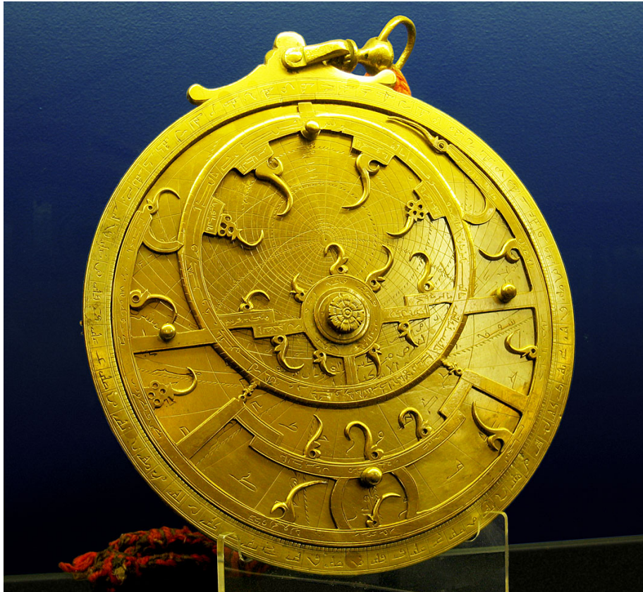
Figure 78. “An 18th Century Persian astrolabe – maker unknown. The points of the curved spikes on the front rete plate, mark the positions of the brightest stars. The name of each star being labeled at the base of each spike. The back plate, or mater is engraved with projected coordinate lines.” From the Whipple Museum of the History of Science in Cambridge. Photograph by Andrew Dunn, 5 November, 2004. http://www.andrewdunnphoto.com/ , accessed December, 2017.
