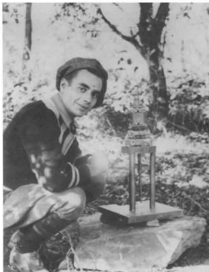
Vic with a Schmidt vertical field magnetic balance, for Gulf, early 1930's.
