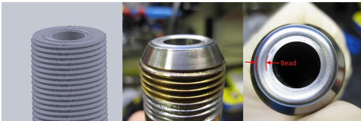
Figure 16. Bead seal design. The schematic (left), the cone-in-cone body adapted to the bead seal with a 1/16^{\text{th}} radius (middle), and the top view of the bead seal (right). The bead design requires a compliant gasket to plastically deform to create the seal.
