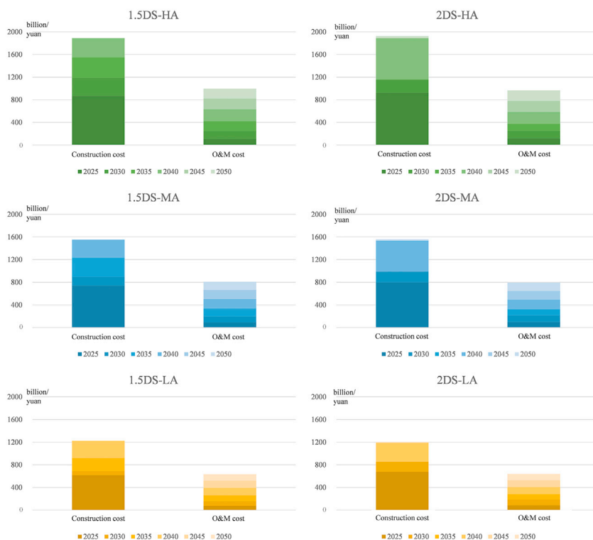
Figure 7. Construction and O&M cost of flow battery to supplement power system adequacy 2DS, 2°C temperature control target scenario; HA, High adequacy scenarios; MA, Medium adequacy scenarios; LA, Low adequacy scenarios.
