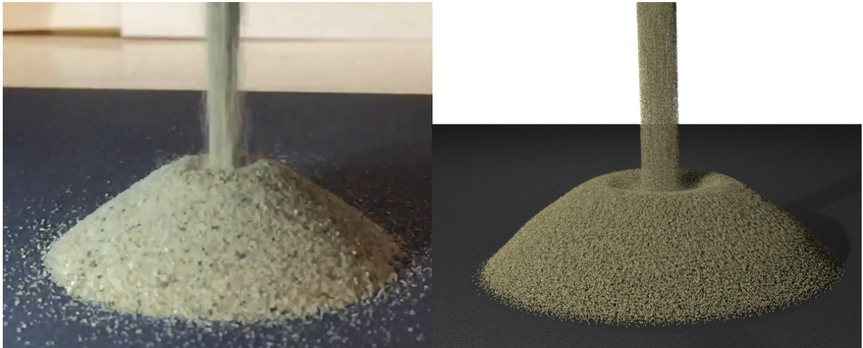
Figure 4.2: Sand is poured from a spout into a pile in a lab (left) and with our method (right)
