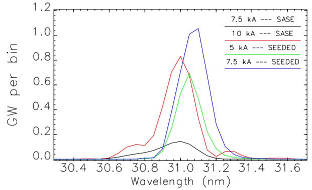
Figure 5: Predicted (GINGER calculations) output spectra at the 31-nm wavelength fundamental for the various SASE and seeded cases. Each bin is 64.6 meV wide while 1 GW is equivalent to  $1.0 \times 10^{13}$  photons.
