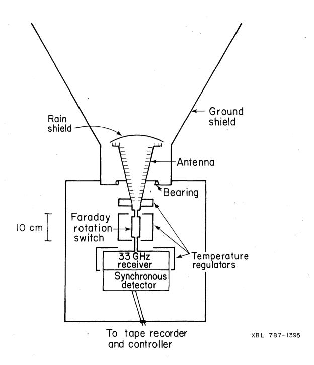
Fig. 1 Schematic of polarimeter
