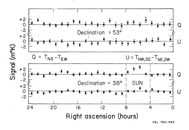
Fig. 2 Measured Stokes parameters Q and U as a function of position in the sky. Data eliminated because of sidelobe contamination by the sun is indicated.
